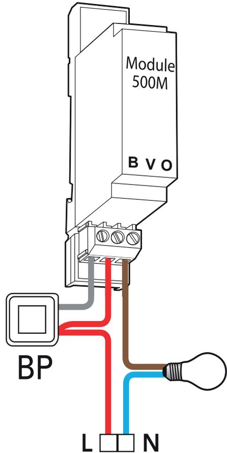
CABLAGE D'UN MODULE 500
